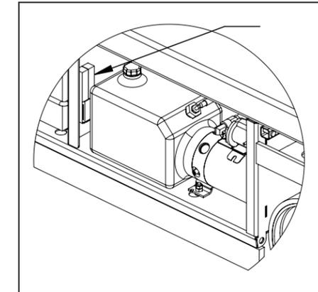
FIGURE 2: Maintenance Lock Pin Storage
