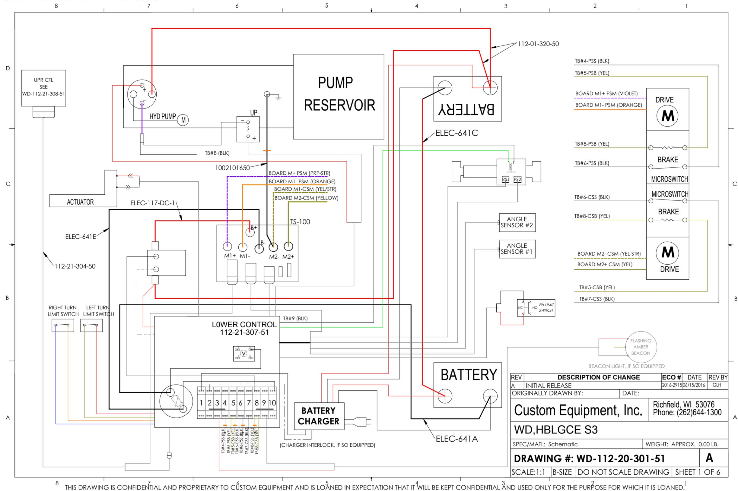
5.2 | LOWER CONTROLS WIRING DIAGRAM WD-112-21-307-51
